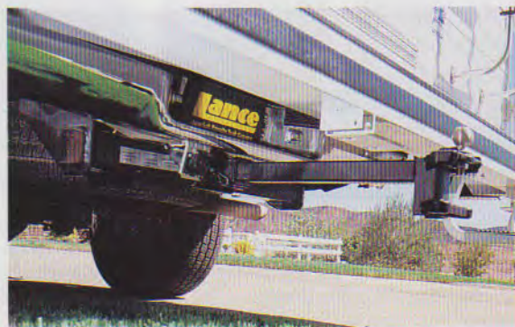
Solid steel extension bar with a weight equalizing hitch.
